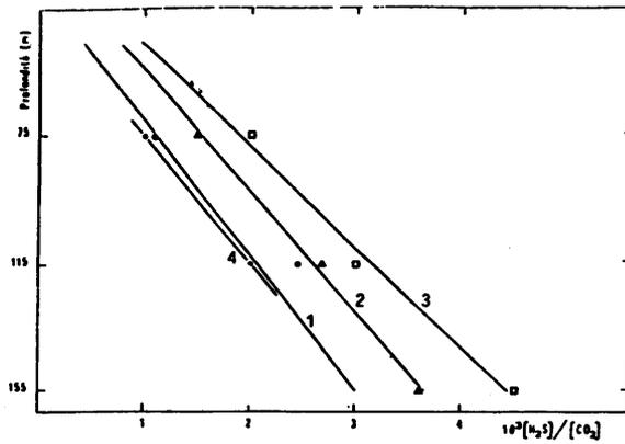
Figure 1: Bagni San Filippo mine. Depth versus  $H_2S/CO_2$  concentration ratio. Straight lines 1, 2 and 3 represent the gradually lowering piezometric level. Line 4 represents flooding in the deepest mining level.
