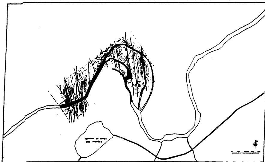
Figure 5. Faults location intersecting the Oeiras River, after seismic geophysics by Nunes de Sousa (1989).
