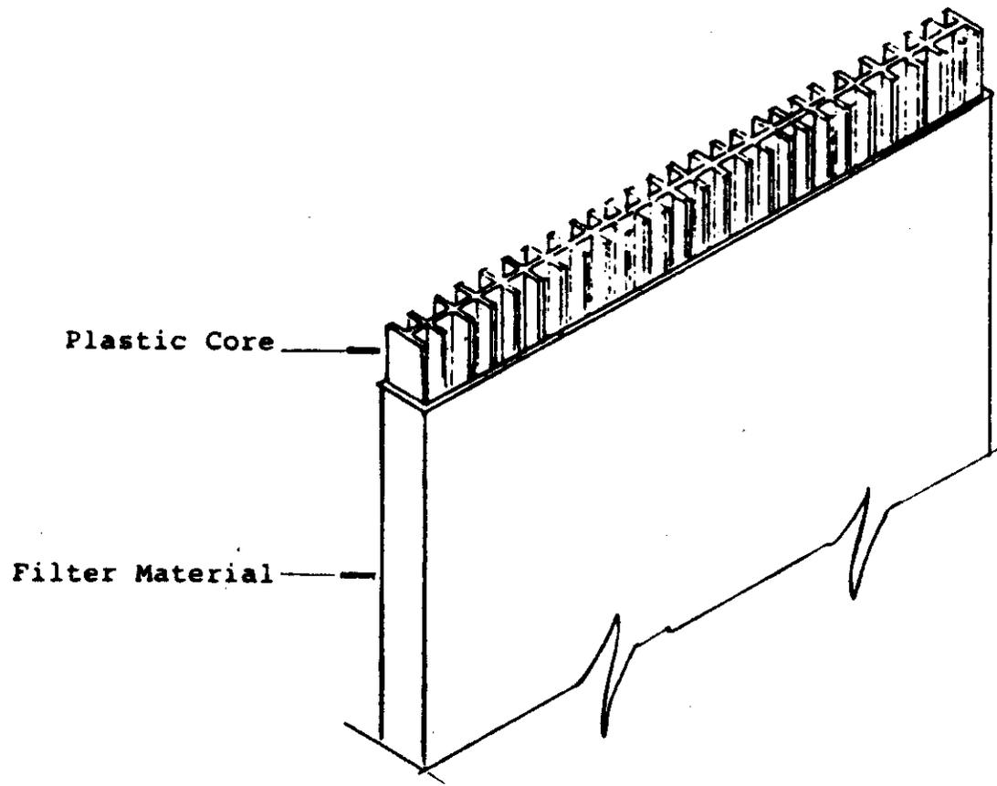
Fig. 1. Prefabricated Wick Drain
