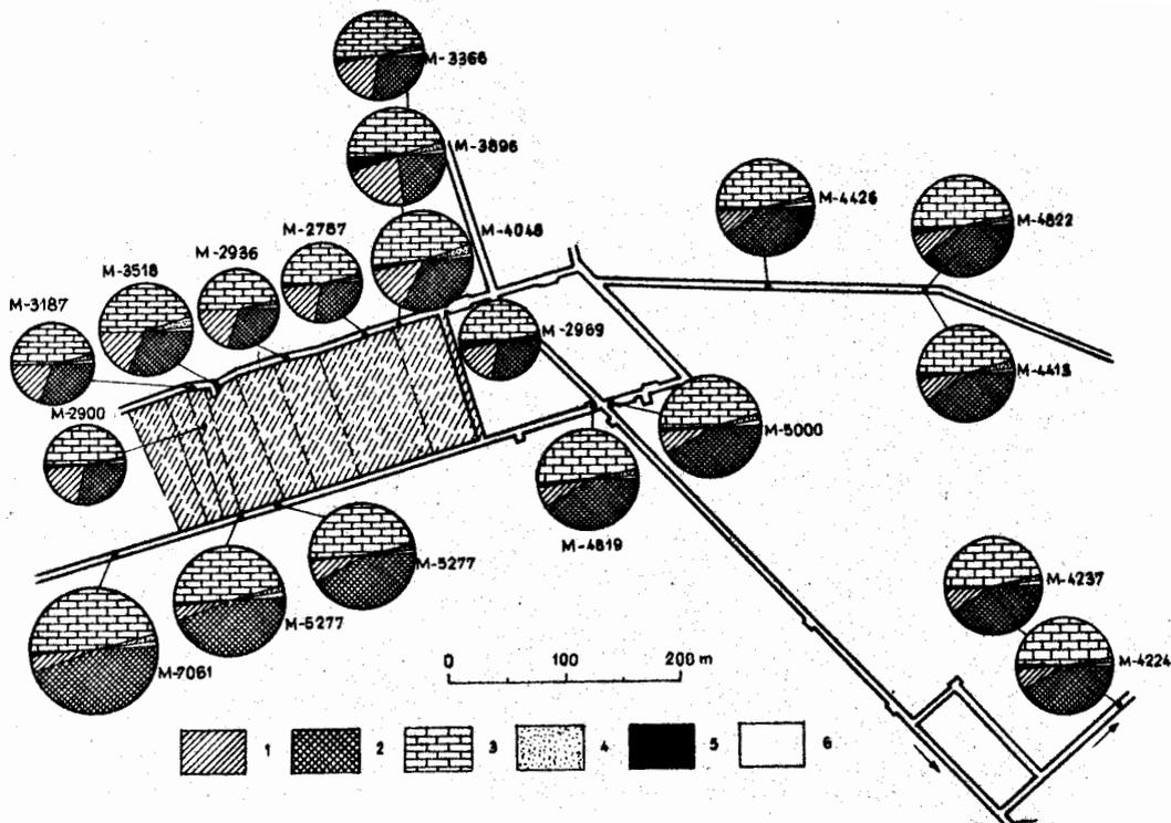
Fig.4. Map of the water chemistry of the inflows of the extraction gallery (longwall) region of the K-1 mine (the level of 920 m) drawn according to the strate in the end of 1983, 1 -  $\text{HCO}_3$ , 2 -  $\text{Cl}$ , 3 -  $\text{Na} + \text{K}$ , 4 -  $\text{Mg}$ , 5 -  $\text{SO}_4$ , 6 -  $\text{Ca}$ .
