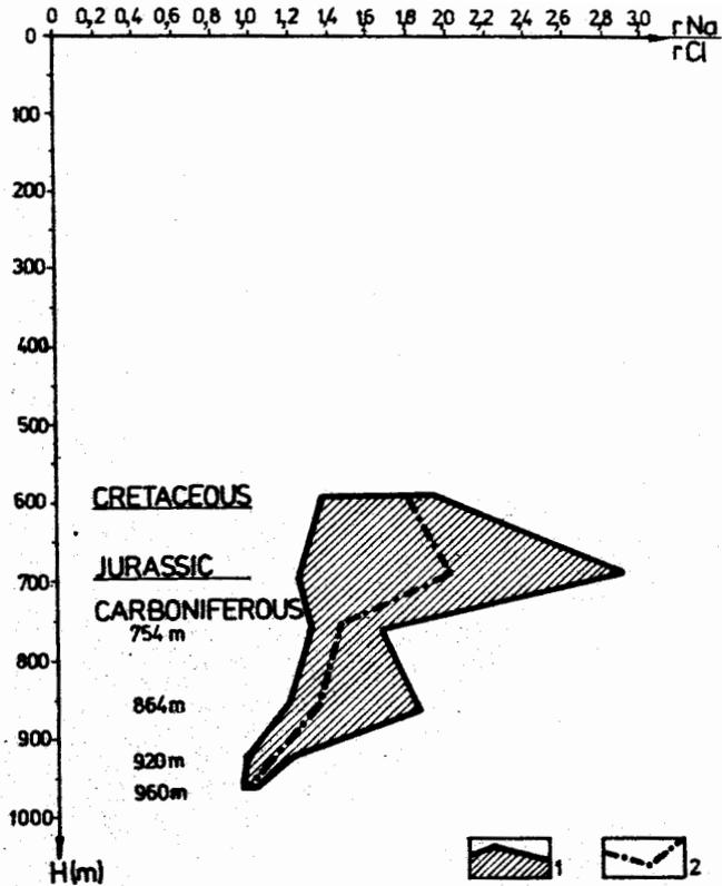
Fig.2. Depth changes in the rNa : rCl value in water inflows of the K-1 mine 1 - area of the alterable index value, 2 - mean index value.
