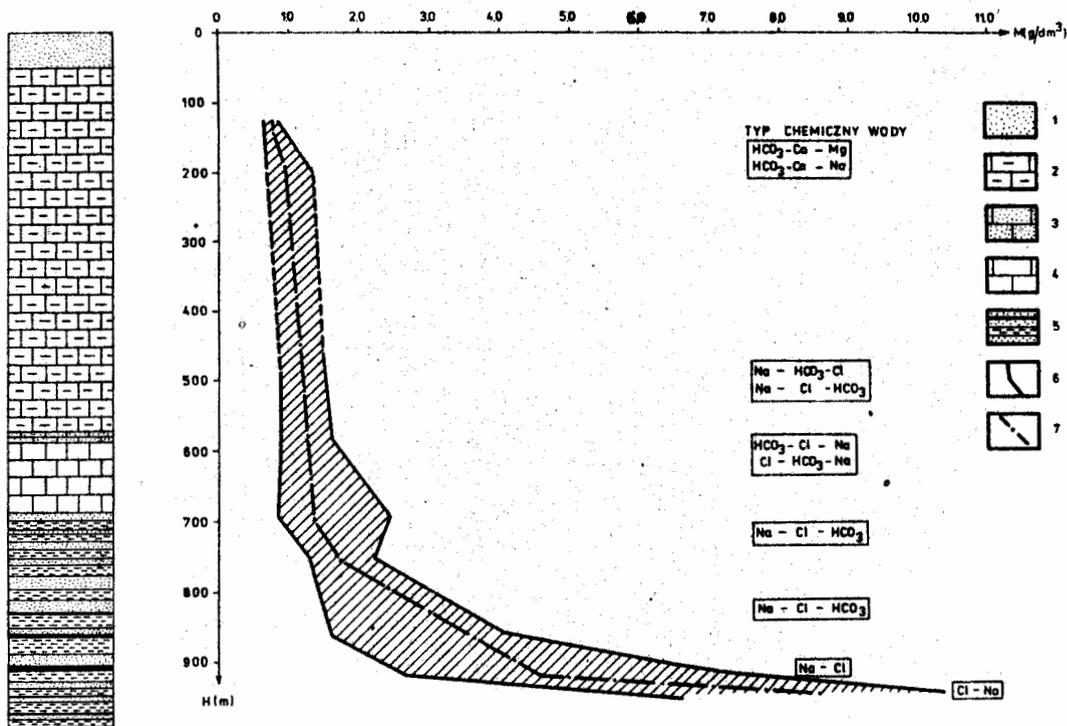
Fig.1. Variations in mineralization and chemical types of the waters of Bogdanka mine with depth
