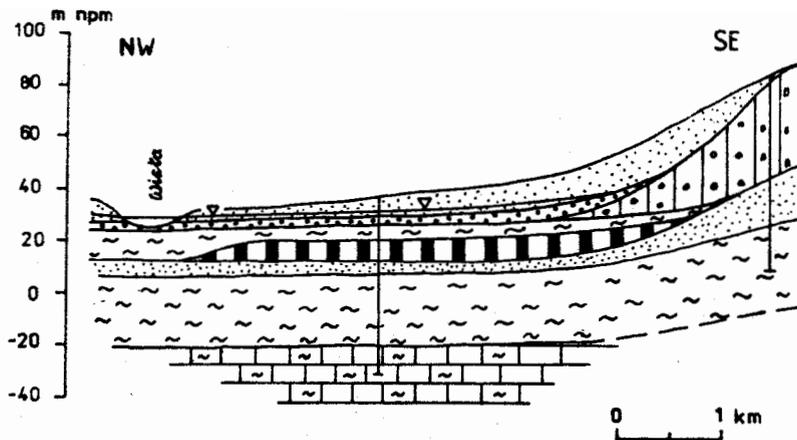
Fig. 4. Hydrogeological profile of the Słonecz-Czarze deposit. Legends as for Fig. 2.
