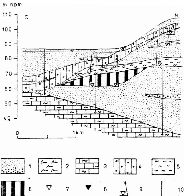
Fig. 2. Hydrogeological profile of the Drzewce deposit.
