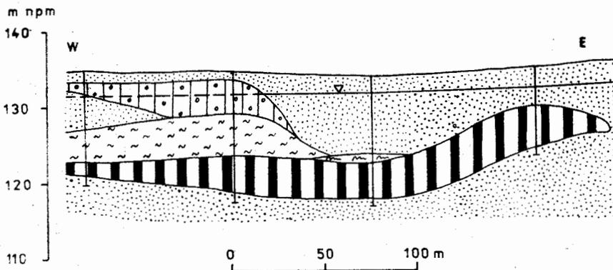
Fig. 5. Hydrogeological profile of eastern part of the Wola Owadowska deposit segment. Legends as for Fig. 2
