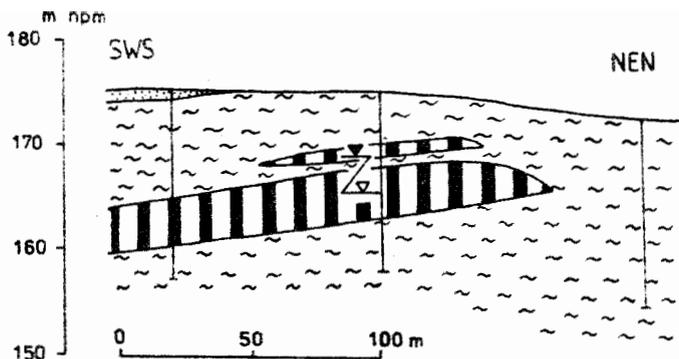
Fig. 3 . Hydrogeological profile of the Polska Nowa Wies deposit segment
