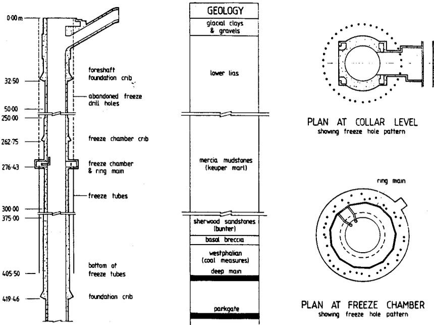
Fig. 3 Schematic Arrangement for Ground Freezing
