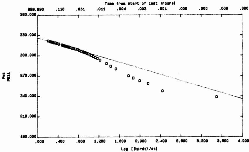
Fig. 5 Asfordby Upcast Shaft: Horner Plot
