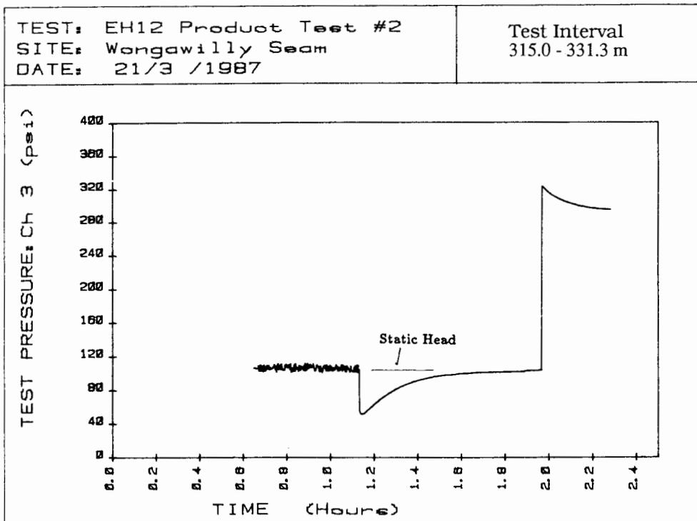
Fig. 5(b). Data from test interval pressure transducer- Hole EH12, Wongawilly Seam
