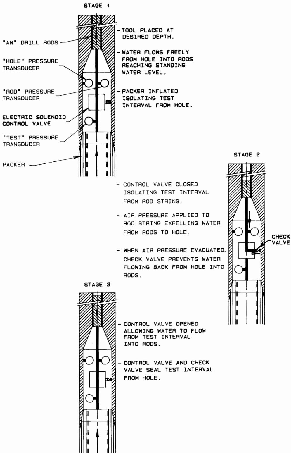
Fig.2. Principle of operation for production test
