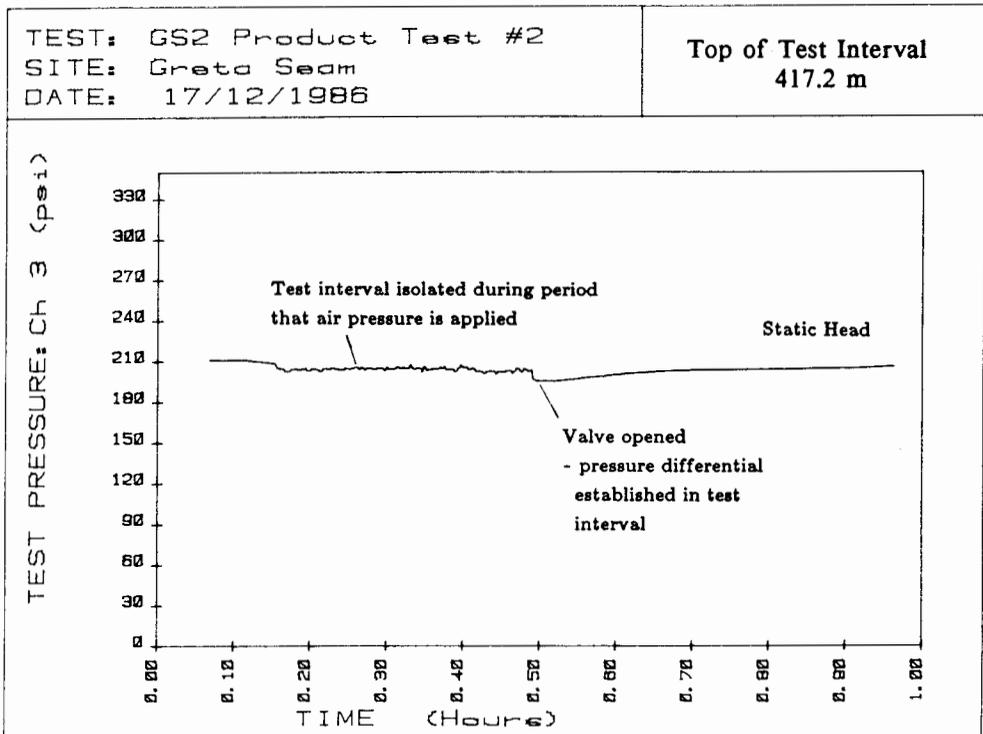
Fig. 4(b). Data from test interval pressure transducer- Hole GS2, Greta Seam
