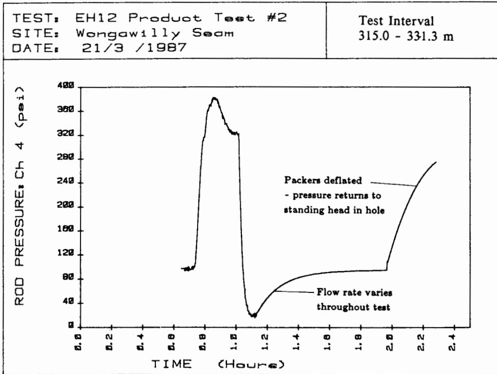
Fig. 5(a). Data from rod-string pressure transducer- Hole EH12, Wongawilly Seam
