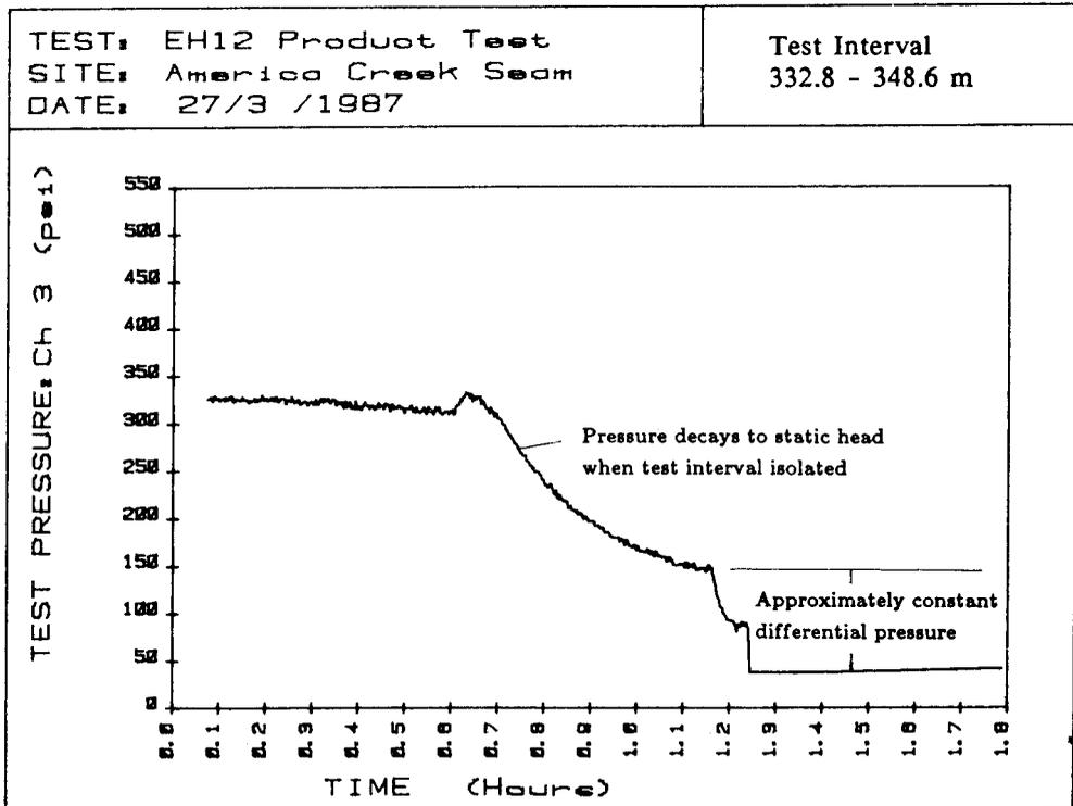
Fig. 6(b) Data from test interval pressure transducer- Hole EH12, American Creek Seam
