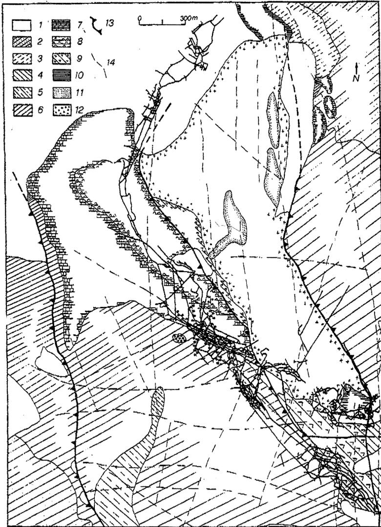
Figure 1. The Gavorrano Underground Pyrite Mine, Tuscany, Italy: Outcrps, faults, fractures and mine network.
