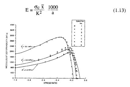
FIGURE 7 - Variation of modulus of deformability with stress ratio,  $k = \sigma_3'/\sigma_1'$ .
