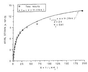
FIGURE 6 - Example of transformed stress-strain curve to determine parameter "a" (specimen No. 8)
