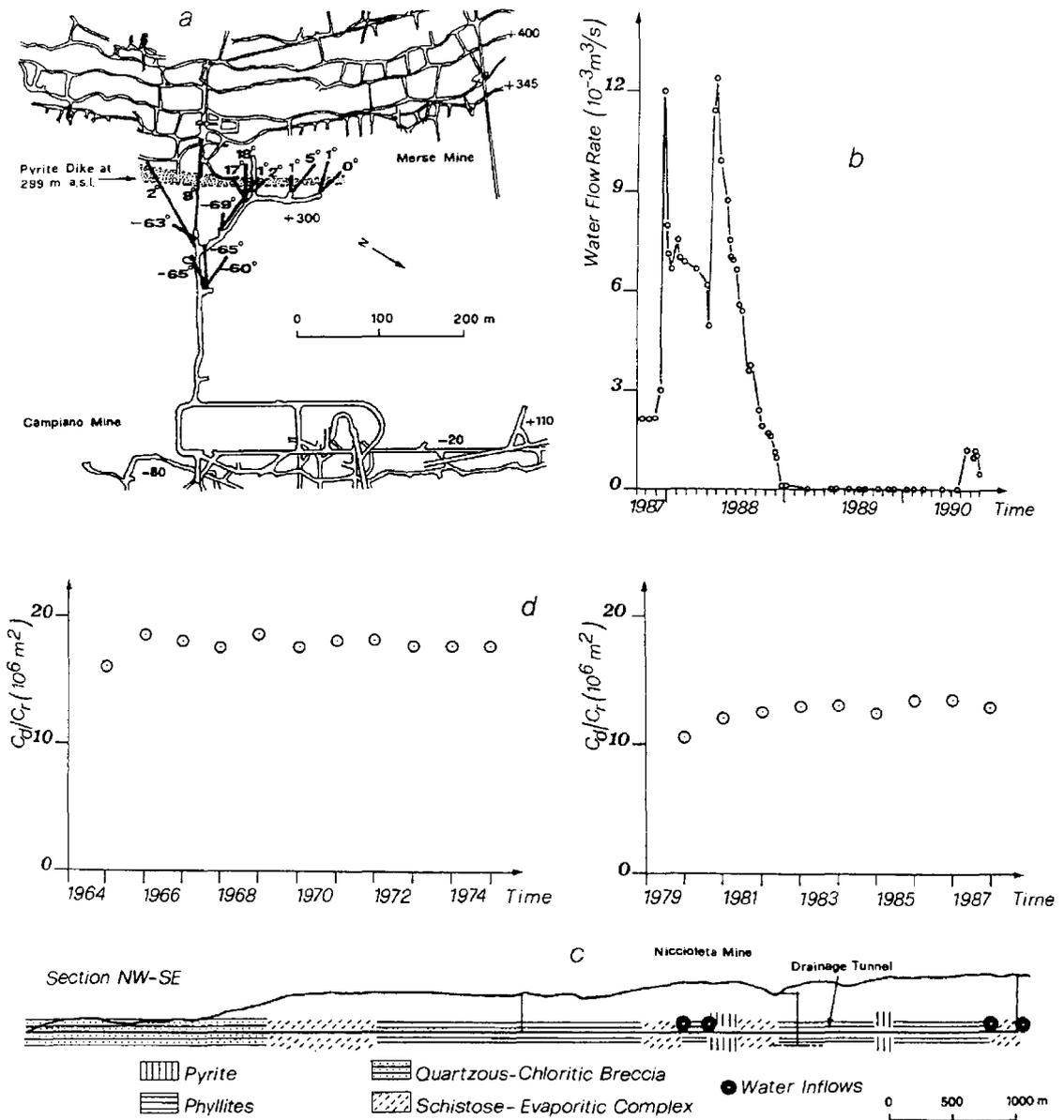
FIGURE 4. Irregularities of water flows drained from mines. Above: drainage system of the Merse mine (a) and flow-rate of the drained water (b). Below: Niccioleta mine (c) and ratio between cumulative quantity of the drainage water and cumulative rainfall (d).
