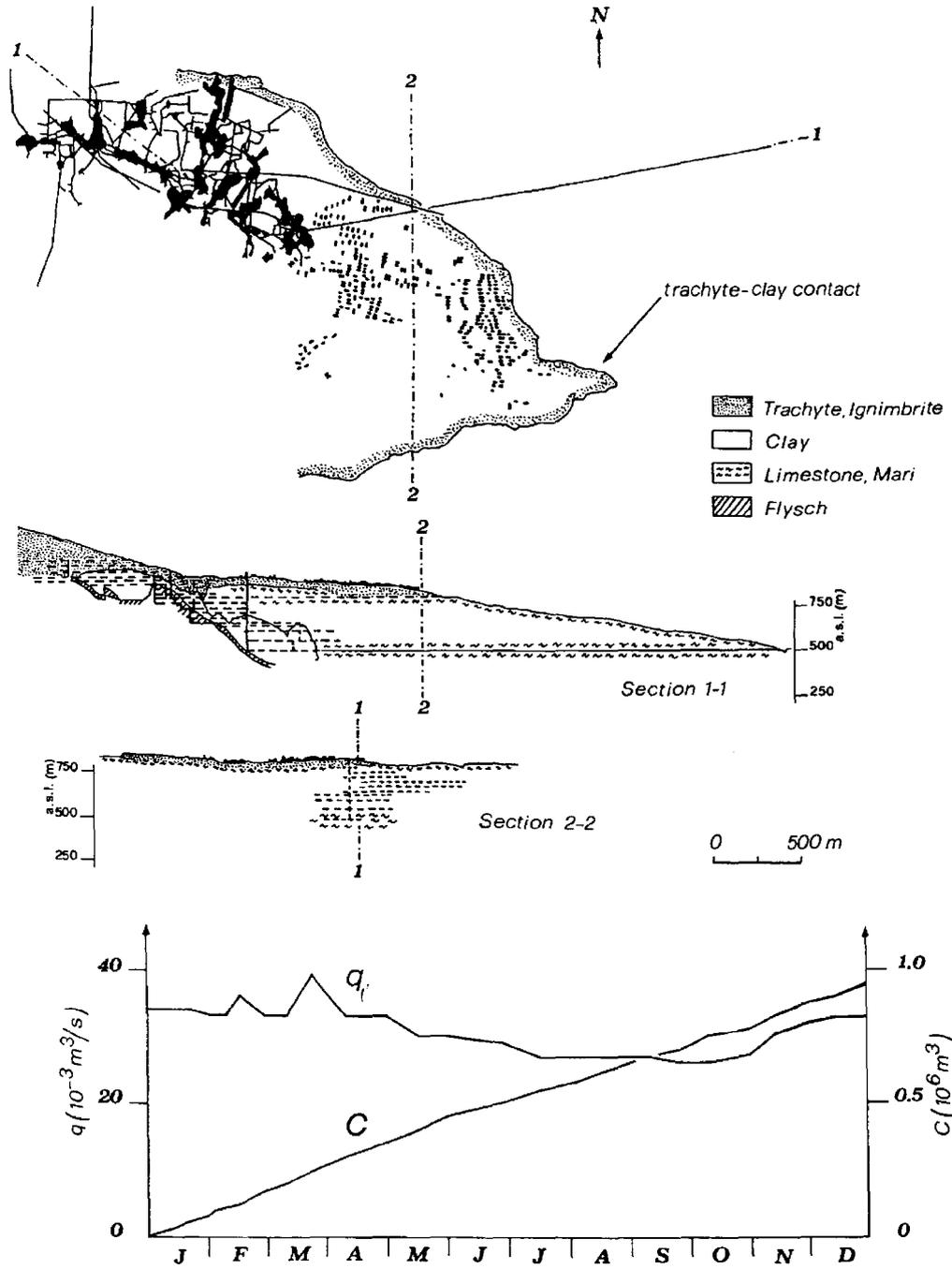
FIGURE 3. Abbazia S. Salvatore Mine. Above: plane and sections of the mine. Below: flow-rate,  $q$ , and cumulative quantity,  $C$ , of water drained from the mine.
