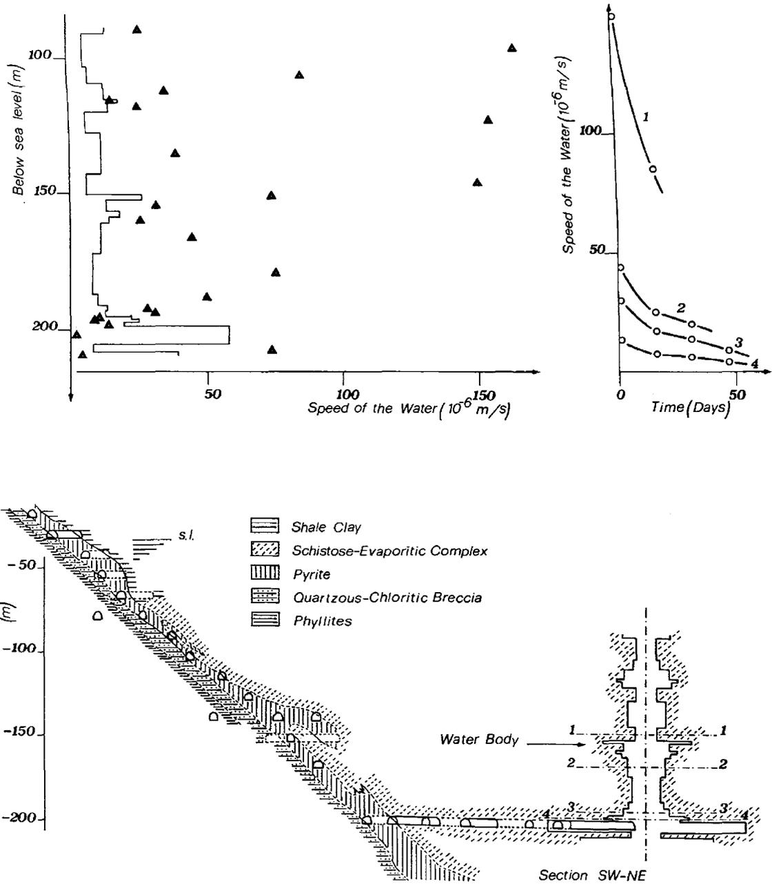
FIGURE 1. Water body detected by means of boreholes in proximity to the hangingwall of the deposit in the Campiano mine. Above: speeds of the water in the body. Below: cross-section of the mine in correspondence to the water body.
