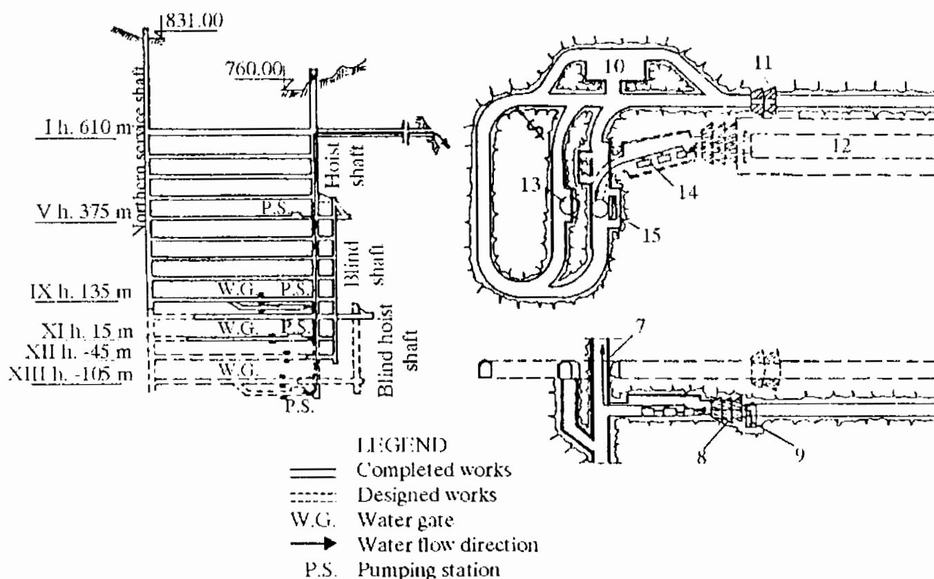
Fig. 3. Mine drainage flow-sheet upon opening of the 13th horizon with drainage facilities layout on the 13th horizon
