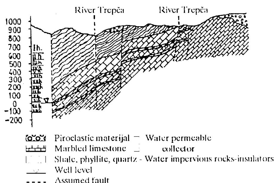
Fig. 2. Predicted hydrogeological profile
