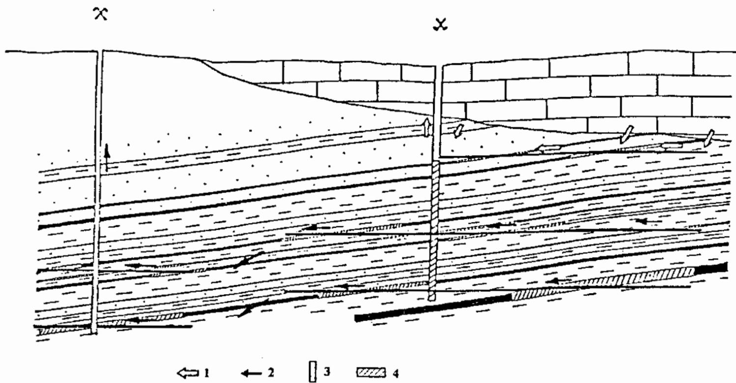
**Fig. 2 Scheme water intake in a partially flooded mine.**
