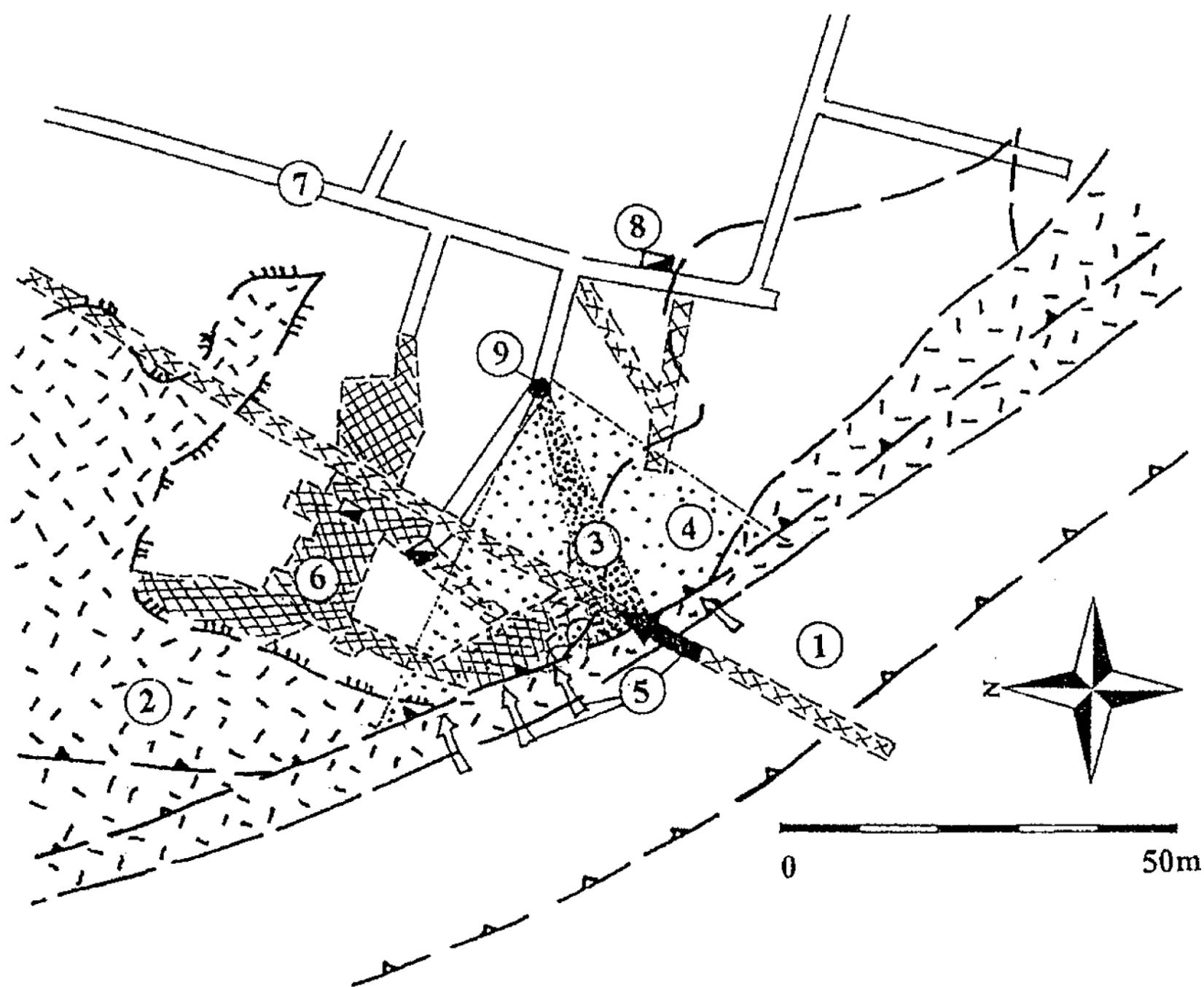
Legend: 1 - pervious layers with karst and fissured porosity, 2 - impervious layers, 3 - narrower injection area, 4 - broader injection area, 5 - foreseen water inflows, 6 - backfills, 7 - galleries, 8 - blind shafts, 9 - fan arrangement of injection boreholes
