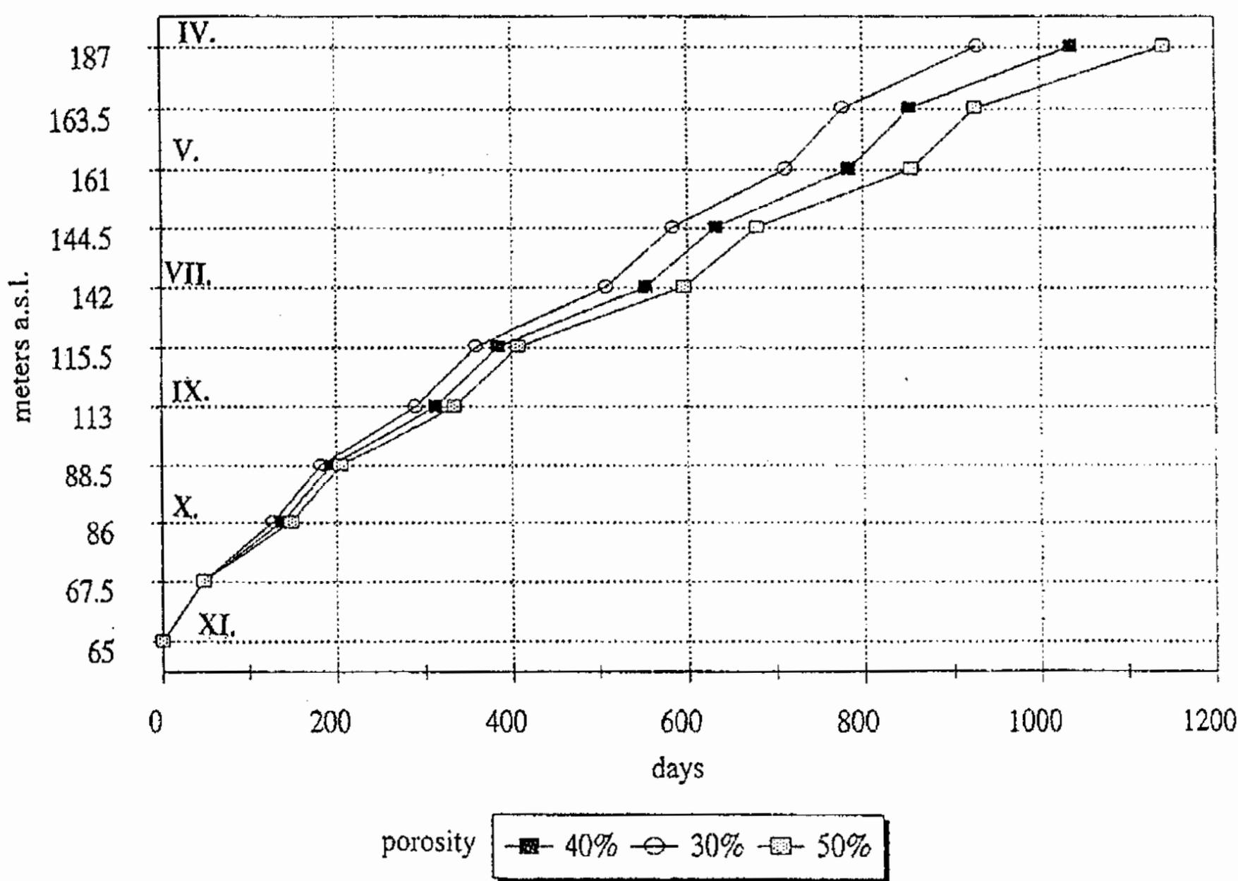
Figure 1: Forecast diagram of flooding the pit between the XIth and IVth levels
