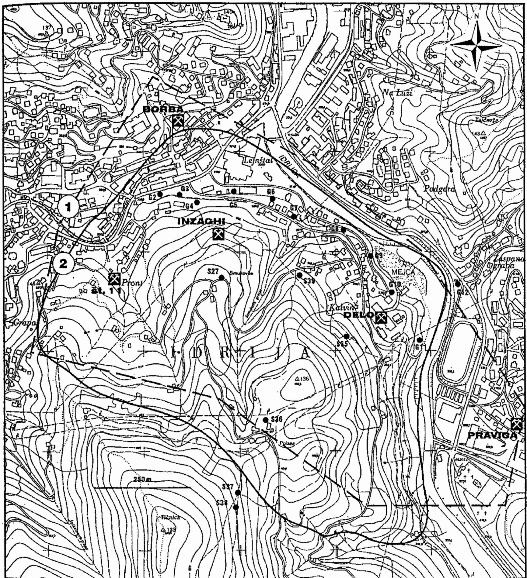
Legend: 1- Extraction area of the Idrija Mercury Mine, 2 - Area influenced by the Idrija Mercury Mine, • G, S - Piezometric/inclinometric boreholes
