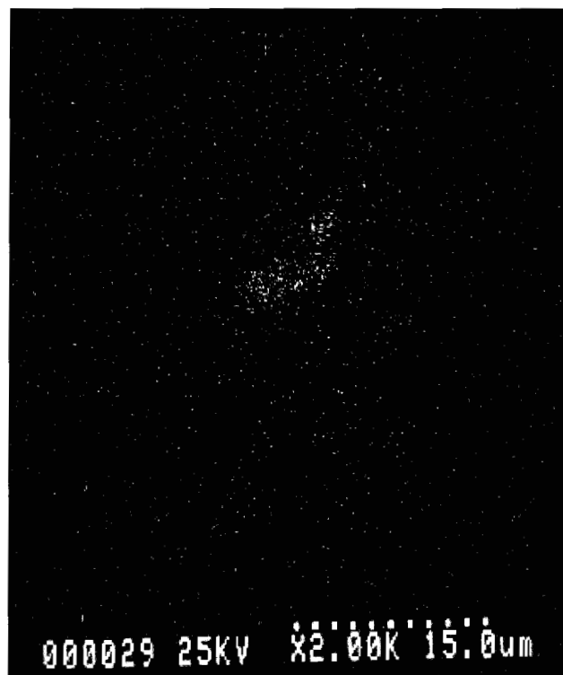
Figure 10. Map of the lead related to the image of the sample in Figure 8: the white dots clustered at the centre indicate the presence of lead.
