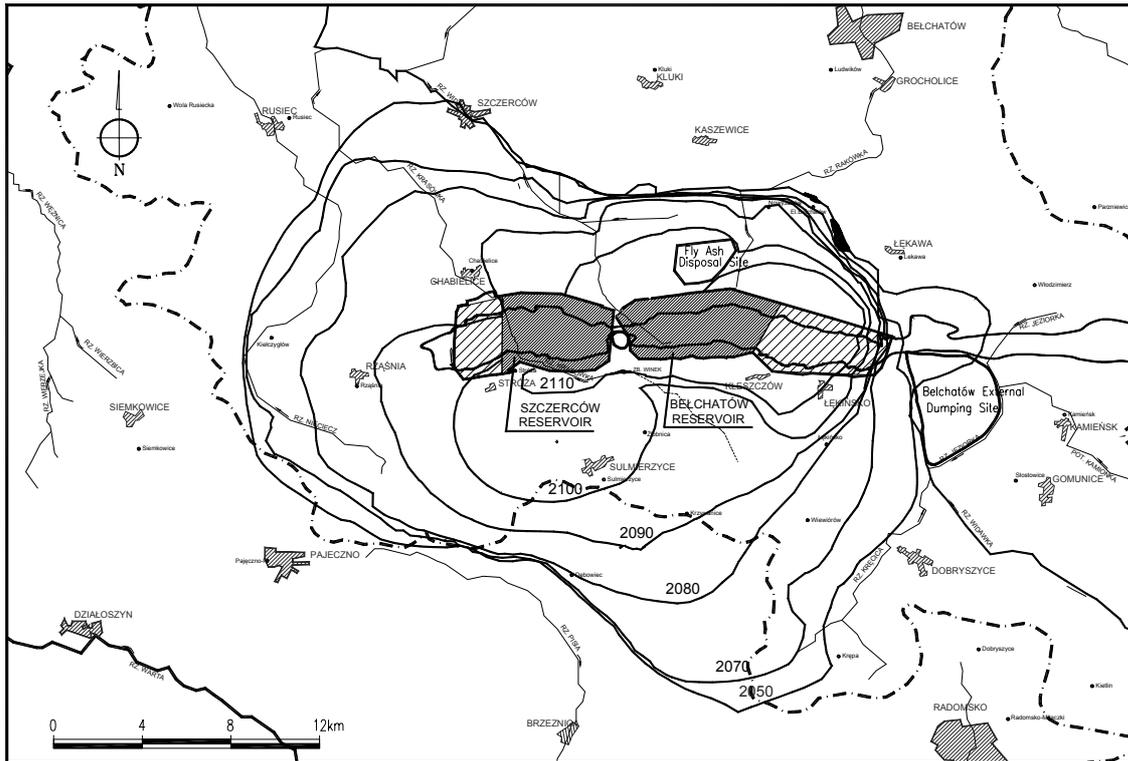
Figure 2. Reduction of the Belchatów mine cone of depression for filling the reservoirs with water in natural way
