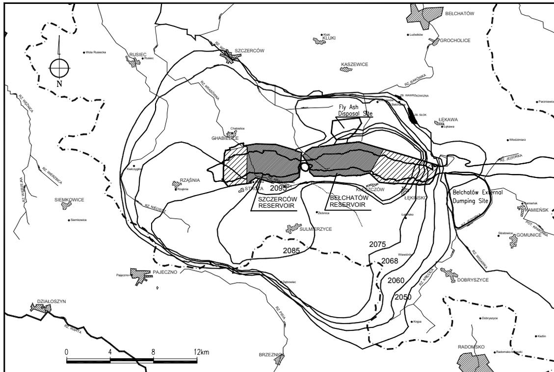
Figure 3. Reduction of the Bełchatów mine cone of depression for filling the reservoirs with water with enhancement of recharge from outside of the cone of depression
