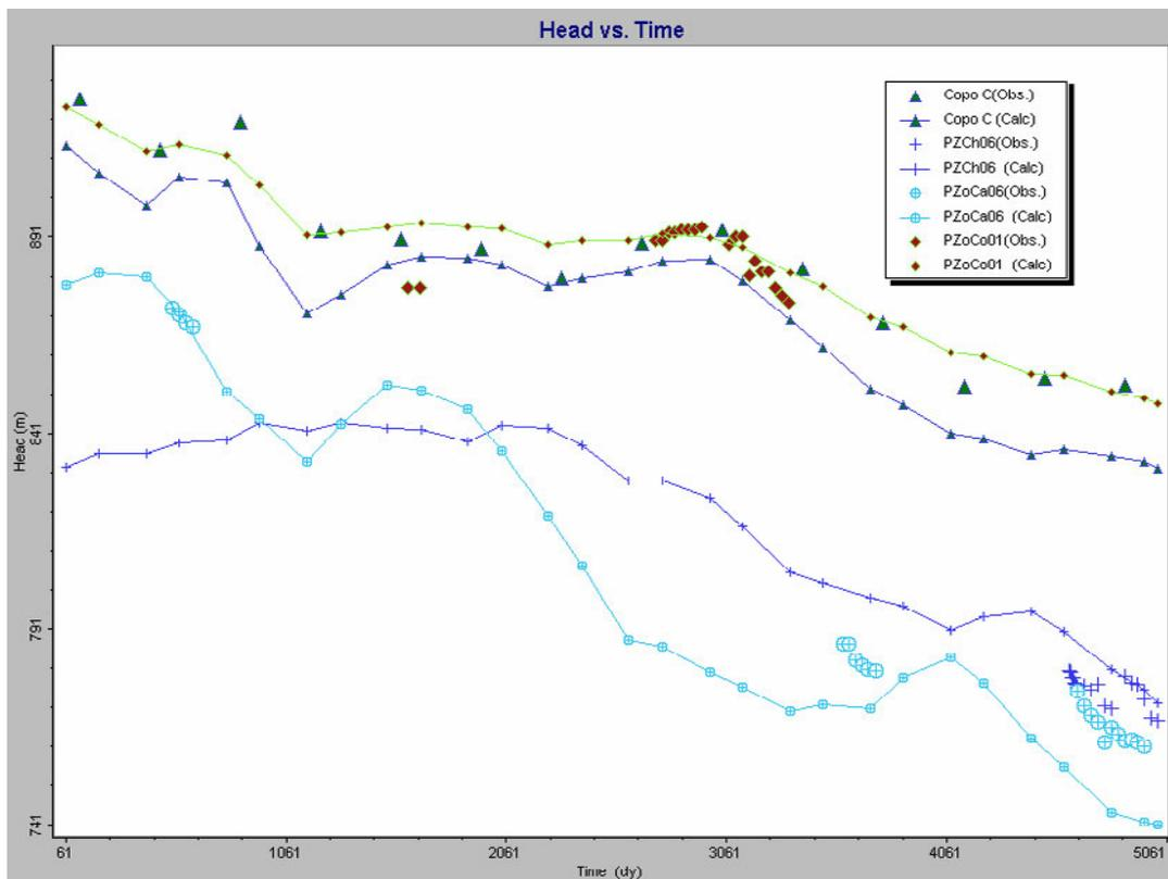
Figure 4: Curves of calibration of the numerical model for some piezometers used in the calibration.
