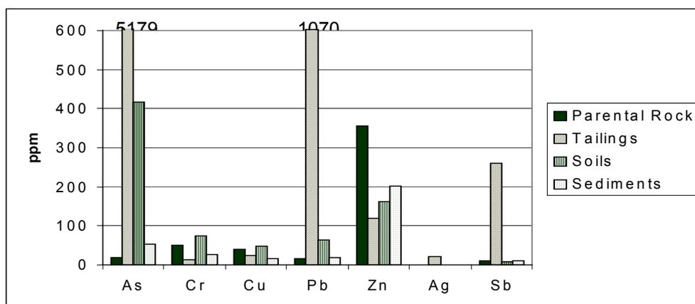
**Figure 2 – Average values of elements (As, Cr, Cu, Pb, Zn, Ag e Sb) in ppm, from parental rock, tailings, soils and sediments (in ppm).**
