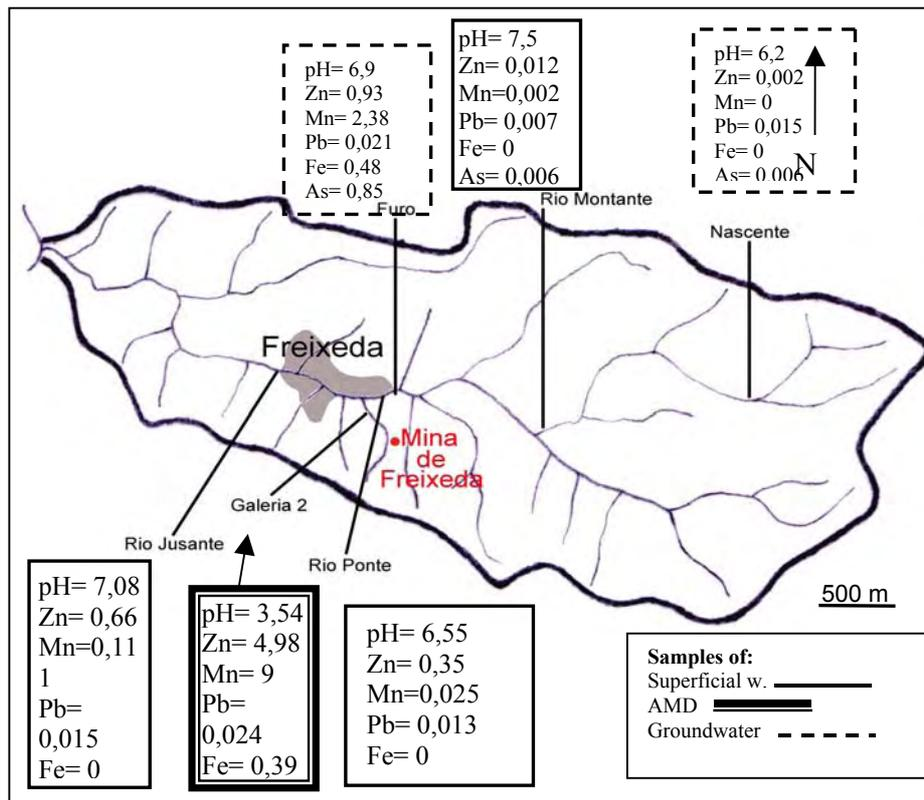
**Figure 4: pH and metals concentration (in mg/l) of water samples from Freixeda. Nascente - Spring; Rio Montante -Rio Ponte-Rio Jusante (superficial water from stream); Galeria 2 - AMD; Furo -well. Quality of water resources**
