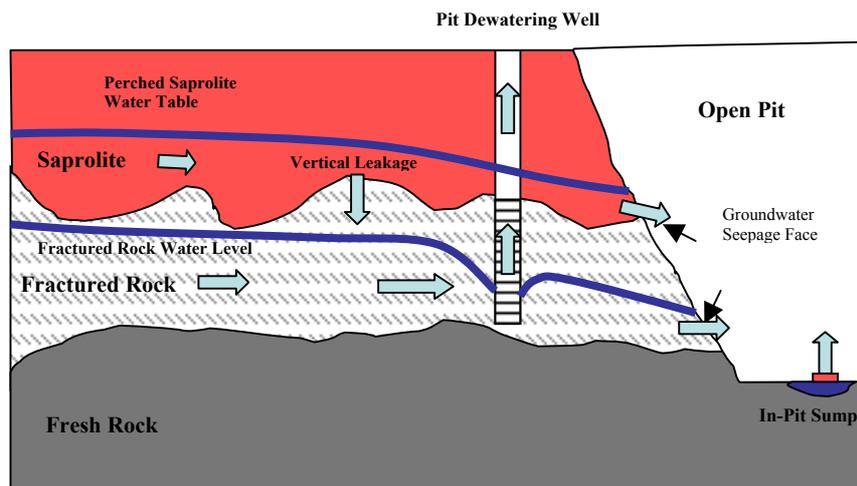
Figure 4: Post-Mining Conceptual Groundwater Flow Schematic
