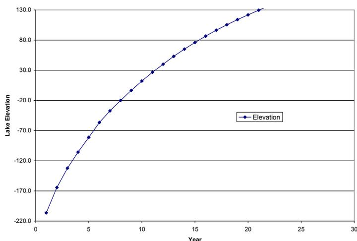
**Figure 7: Post-Closure Pit Lake Filling Curve**
