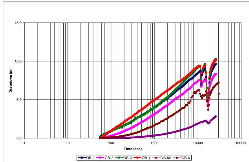
Figure 3: Semi-Log Plot of Drawdown vs Time – PW-1, High Flow Aquifer Test
