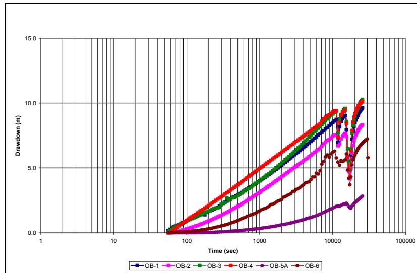
Figure 3: Semi-Log Plot of Drawdown vs Time – PW-1, High Flow Aquifer Test
