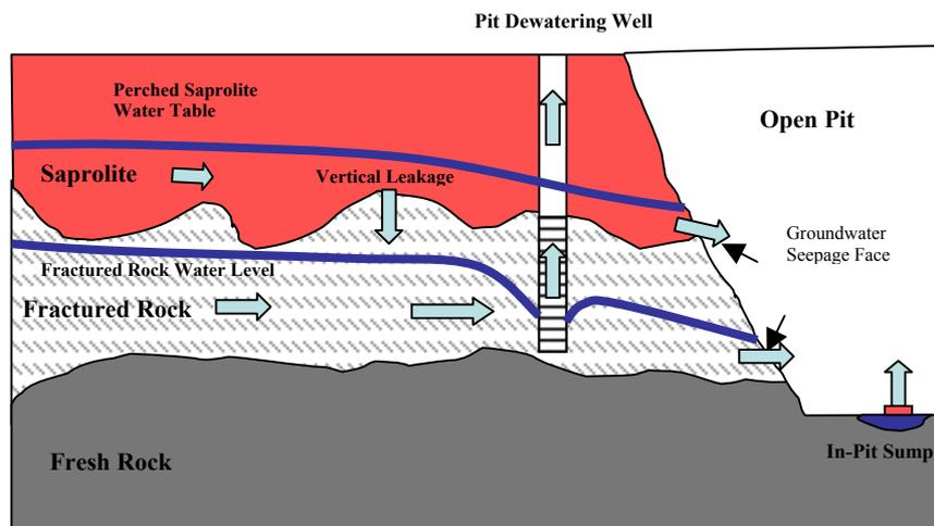
Figure 4: Post-Mining Conceptual Groundwater Flow Schematic
