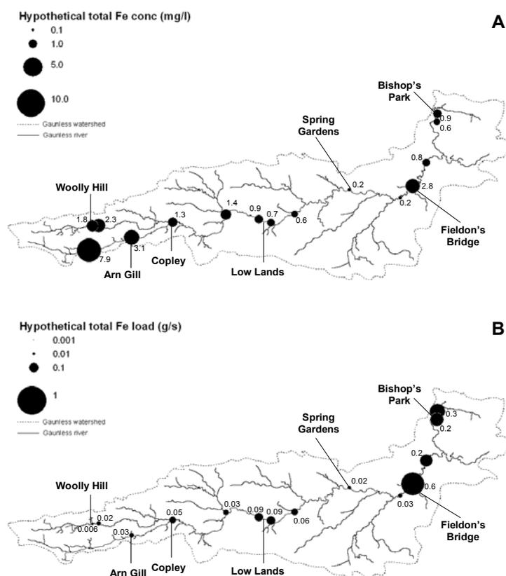
**Figure 3: Hypothetical total iron concentrations (Fig 3a) and total iron loadings (Fig 3b) under low flow conditions with remediation of point mine waters at Low Lands, St Helen Auckland and Bishop's Park.**
