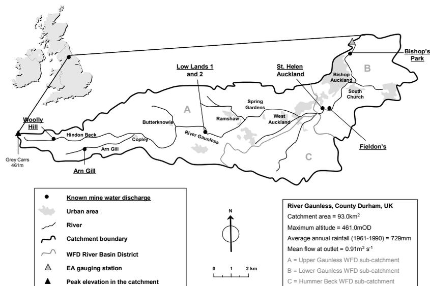
**Figure 1: Schematic map of the Gaunless catchment highlighting known point mine water discharges, urban areas and WFD management boundaries.**
