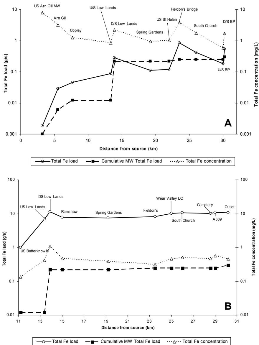
**Figure 2: Total iron load and concentration profiles in the River Gaunless under low flow (Fig 2a) and high flow (Fig 2b: updated from Younger, 2000) conditions. (Note the differing horizontal axis in the two plots).**
