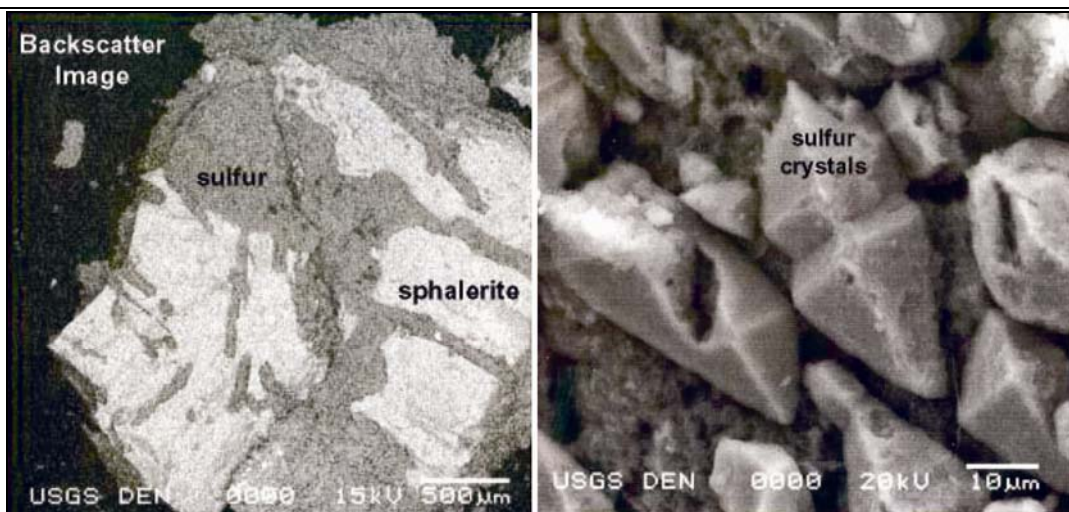
Figure 6. A. Backscatter scanning electron photomicrograph showing the alteration of a sphalerite grain to elemental sulfur, Lower Chatauqua. B. Scanning electron photomicrograph of sulfur crystals, some etched on the surface of pitted and altered sphalerite grain.
