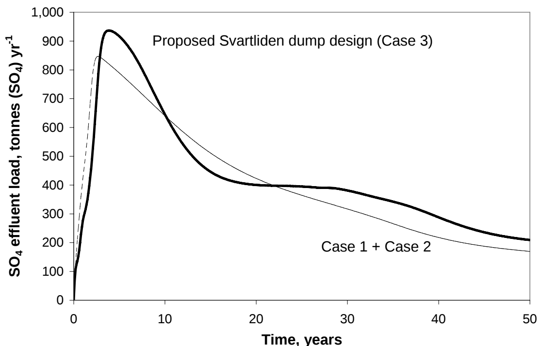
Figure 12. Calculated \text{SO}_4^{2-} load in dump effluent, as a function of time (up to 50 years): A comparison of Case 3 (based on the planned Svartliden dump design) with the combined load expected from two individual dumps containing LC PAF (Case 1) and PAF (Case 2).
