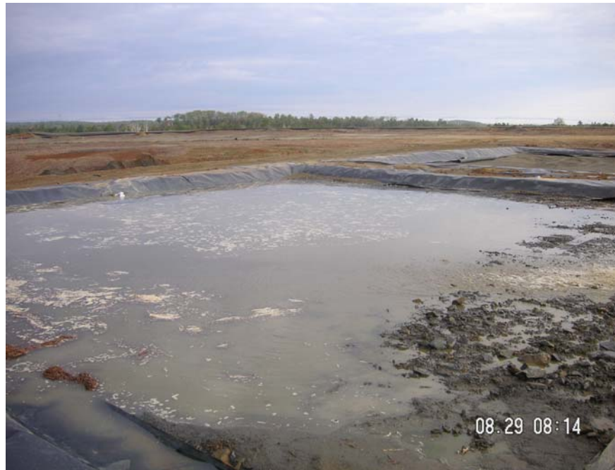
Figure 5. Lysimeter L2 immediately after flooding.
