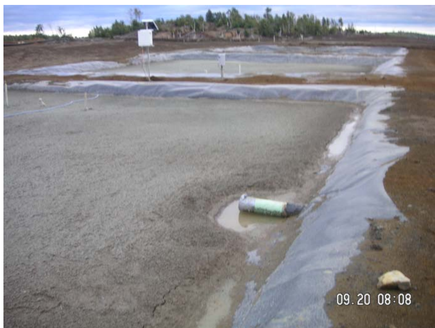
Figure 6. Lysimeter L3 with the topsoil cover.
