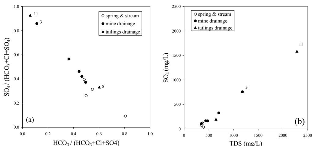
**Figure 2. Dissolved bicarbonate versus sulphate, both normalized to the sum of major anions (a), and sulphate versus total dissolved solids, TDS (b).**
