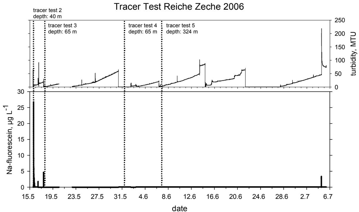
**Figure 3. Results of the 4 Reiche Zeche mine water tracer tests conducted in 2006. Tracer could only be detected for the Tracertest 2.**
