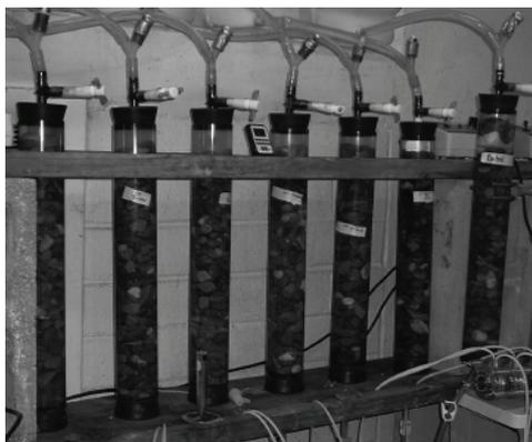
**Figure 2. Experimental columns.**
