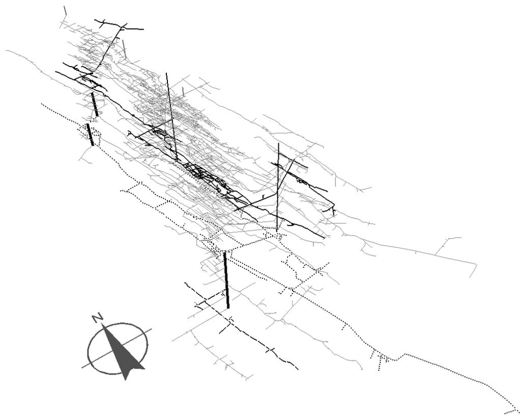
Figure 3. Mine workings scheme in ArcGIS – Olsi – Drahonin Mine
