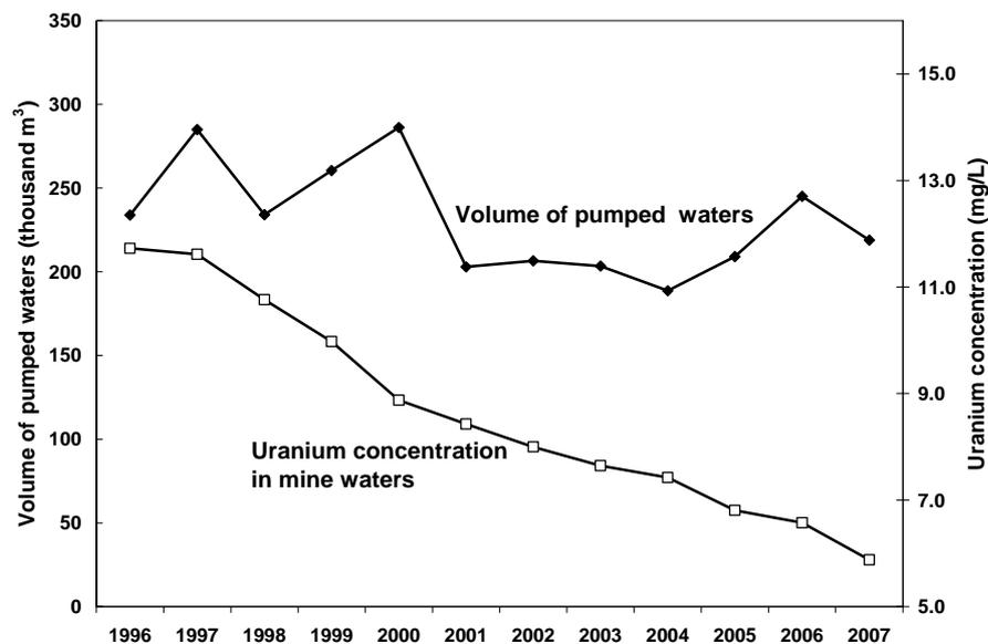
Figure 1. Amount of mine water and uranium concentration in mine waters drained from the flooded Olší – Drahonín deposit to the purification plant
