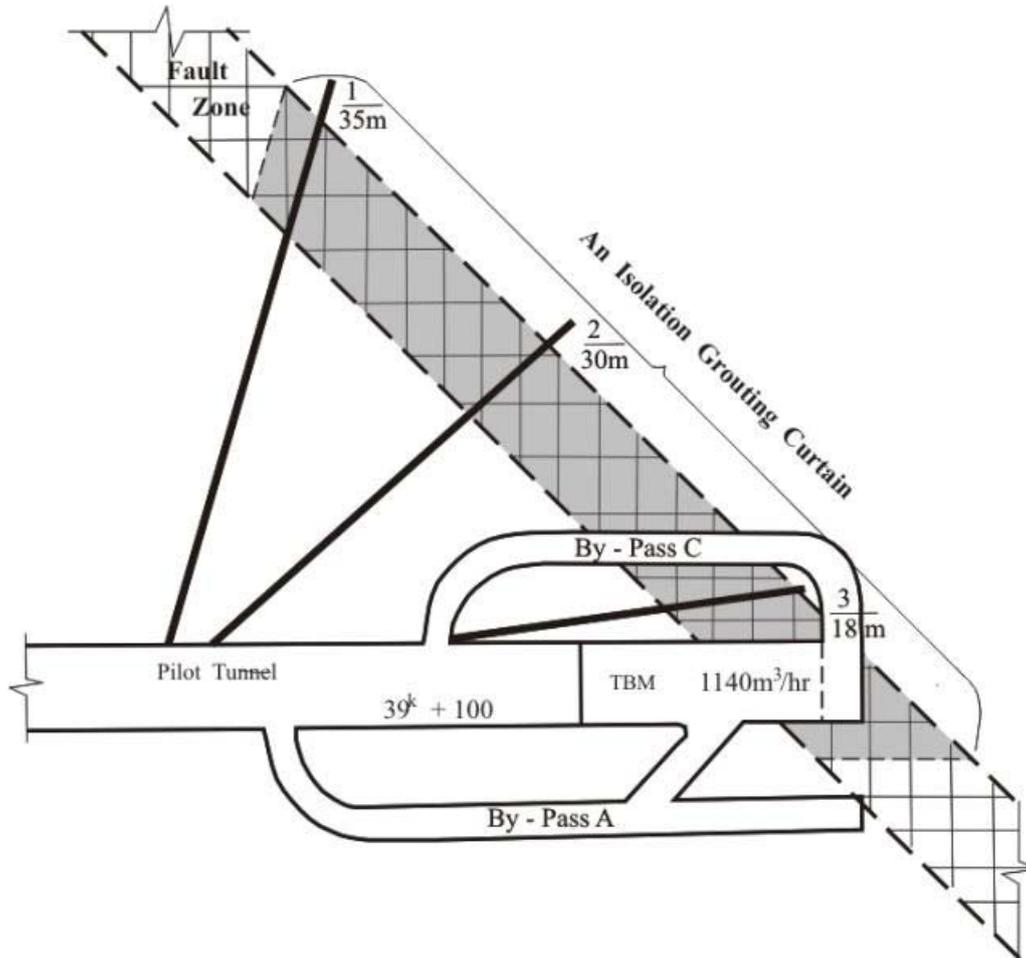
Fig.3 Arrangement of grouting boreholes for elimination sudden inrush of water into Pin Lin Pilot Tunnel
