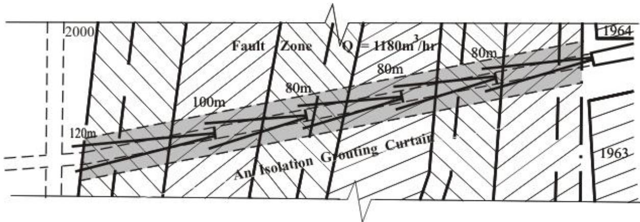
Fig.2 Schematic arrangement of grouting boreholes for ground treatment of water-bearing fault zones at crosscut No 6 of Radyanska coal Mine, Ukraine
