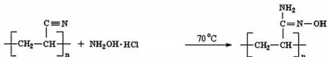
Figure 1. Reaction of hydroxylamine hydrochloride with PAN nitrile group.
