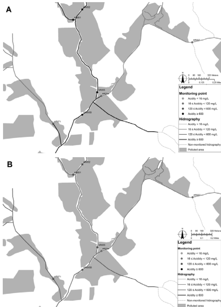
Figure 4 Cartographic representation of the results of the 13 th (A) and 20 th (B) monitoring campaigns for the parameter acidity in a river length of Ararangua watershed
