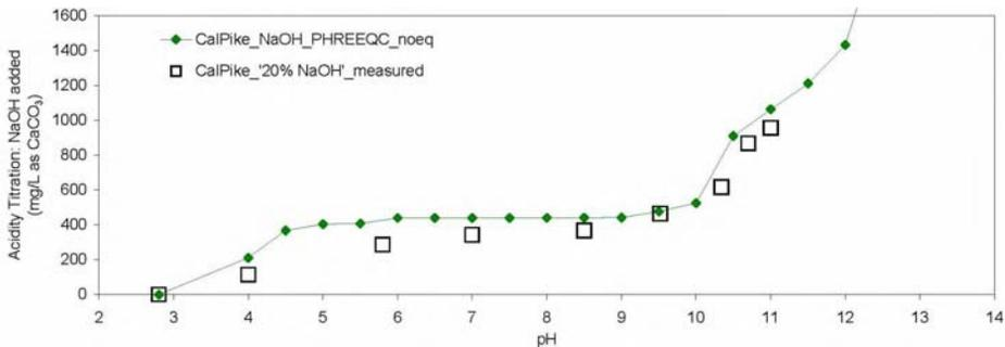
**Figure 1** Data for titration of “Cal Pike” effluent with NaOH at 16 °C. Measured (open symbols) and simulated (filled symbols) values for amount of NaOH added, as  $\text{CaCO}_3$  equivalent concentration, and corresponding pH. Measured titration used 20 % liquid caustic solution
