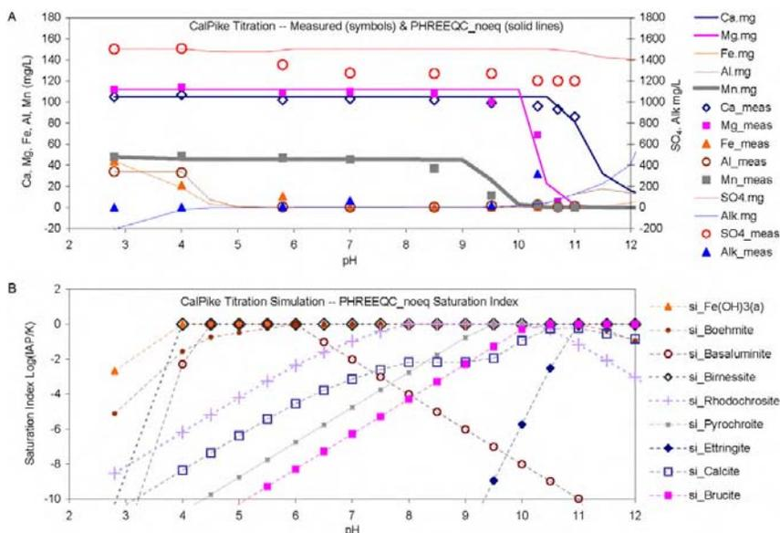
Figure 2 A, Data for measured (symbols) and simulated (solid lines) titration of “Cal Pike” effluent with NaOH at 16 °C without gas exchange. B, Saturation indices for minerals and other solids as a function of pH for simulated solutions
