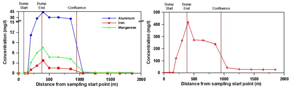
Figure 4 Metals and Sulfate concentration along the sampling length, (left: metals, right: sulfate)
