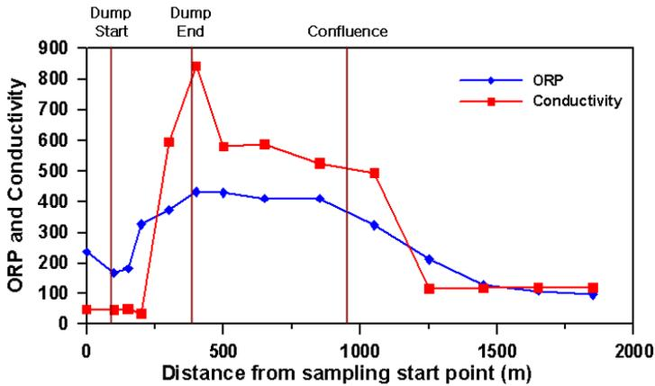
Figure 3 ORP(mV) and Conductivity (µs/cm) along the sampling length
