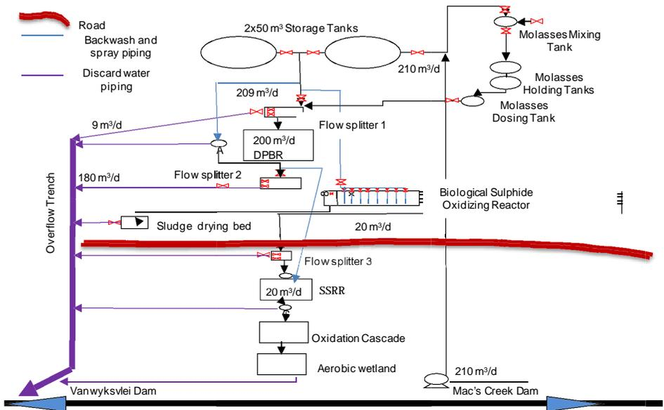
Figure 2 Schematic representation of the IMPI process
