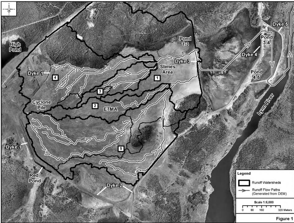
Figure 1 Major watersheds of ETMA and flow directions and based on “raindrop” analysis of DEM
