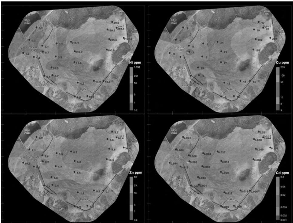
Figure 2 Distribution of soluble metals on the surface of the tailings
