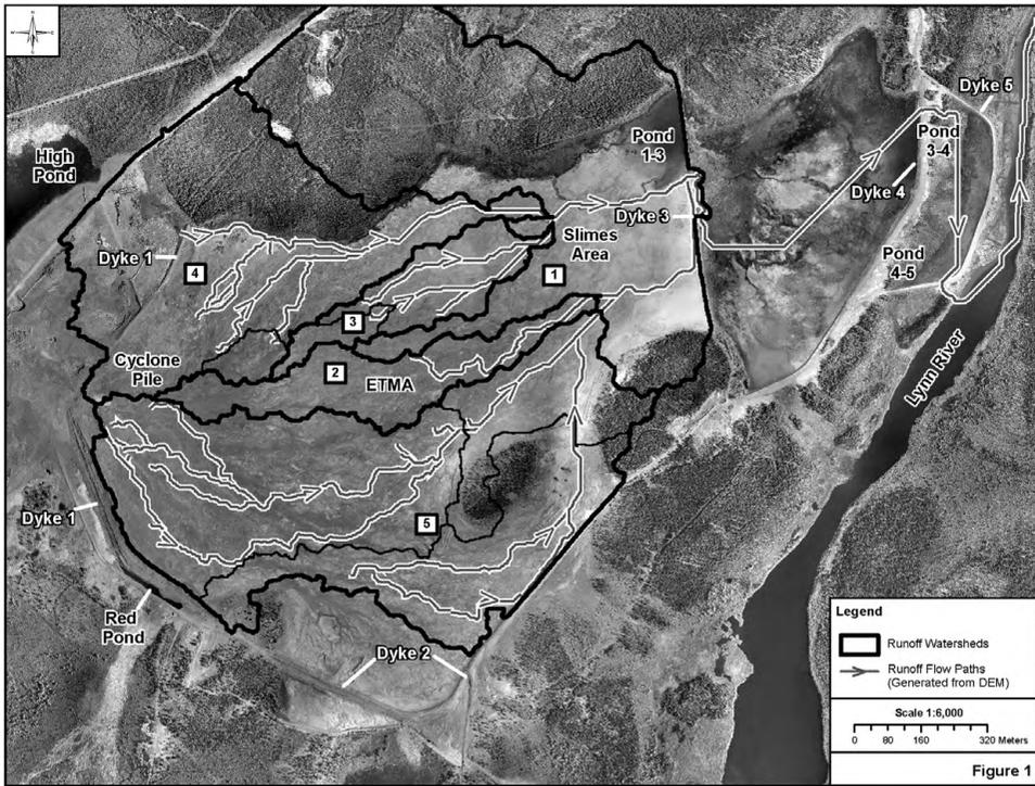
Figure 1 Major watersheds of ETMA and flow directions and based on “raindrop” analysis of DEM
