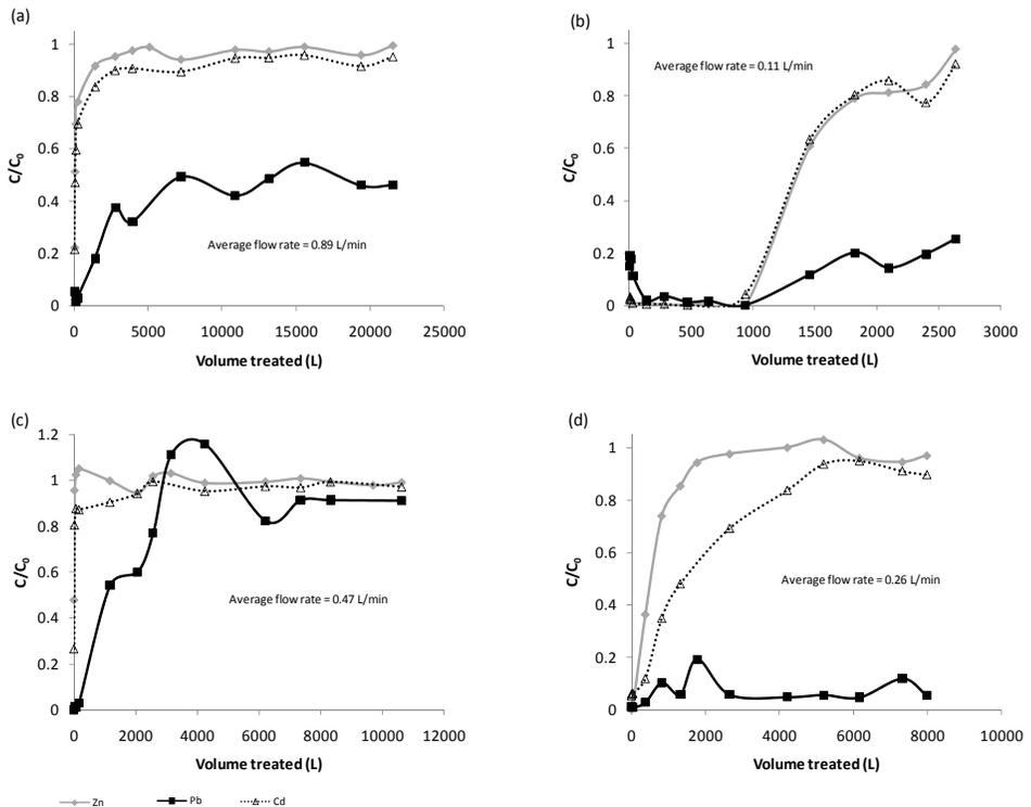
**Figure 2** Removal of Zn, Pb and Cd by (a) waste shell material; (b) peat fly ash; (c) BOS slag and (d) compost, where  $C_0$  = influent concentration and  $C$  = effluent concentration. Average influent concentrations are: Zn = 23.5 mg/L, Pb = 0.5 mg/L and Cd = 0.05 mg/L
