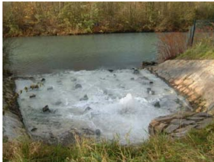
Figure 2 Rapid precipitation of white native sulphur upon aeration of deep, anoxic, hydrogen sulphide-bearing mine waters pumped from approximately 500m depth in the flooded workings of the former Schachtanlage Robert Müser colliery, Ruhr Valley, Germany
