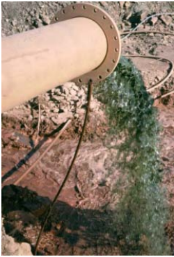
Figure 3 Formation of green suspended sediment of ferrous hydroxide by abrupt neutralisation of acidic mine water at Wheal Jane mine, Cornwall
