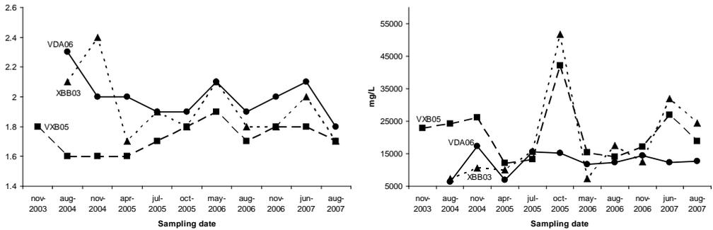
**Figure 3** Time variations of pH and TDS values recorded for the most acidic samples of the waste rock type: VDA06-dacite, VXB05-vent breccia and XBB03-black breccia.
