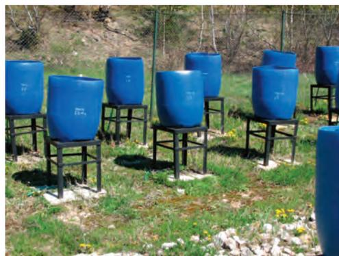
**Figure 2** Emplacement of the barrels used in field-based leaching test.
