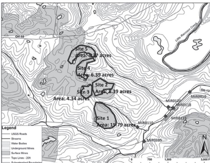
*Figure 2* Non-grid composite soil samples were collected at five strip-mined sites in the Middleton Run watershed for lab leachate analysis. Sites are labelled by number and acreage.
