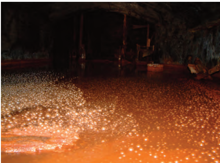
Figure 5 Weidtmans Schacht Merkur mine: degassing of carbonic acid
