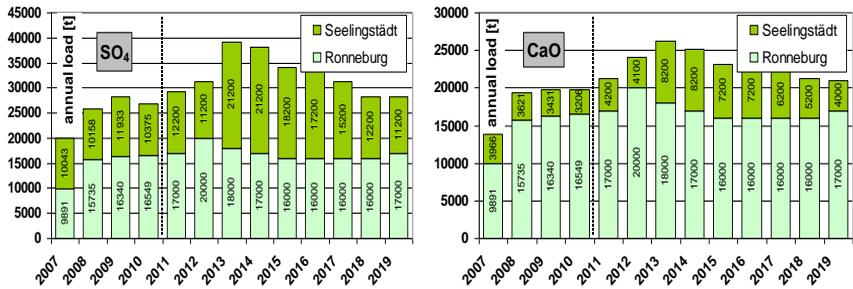
**Figure 2** Measured and predicted released loads of sulphate and hardness (as CaO) based on the planned remediation progress
