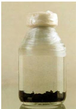
**Figure 1** Photography showing the strong black precipitate that is produced associated to sulphate-reducing bacteria development.
