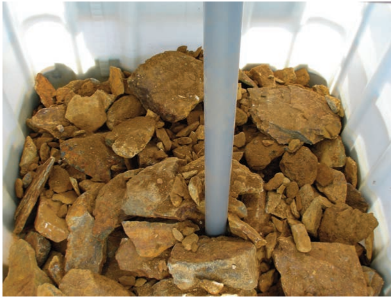
Fig. 1 Illustration of the plastic pipe used for gravity injection of fly ash suspensions into the coarse waste rock fraction.
