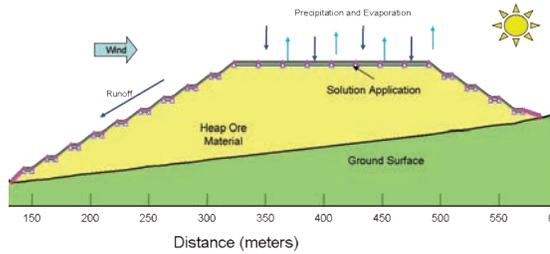
**Fig. 2** Conceptual model schematic.
