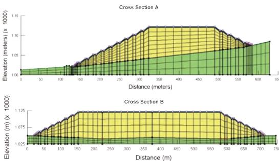
**Fig. 1** Facility cross-sections and model construction.
