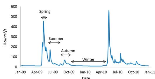
Fig. 2 Typical annual flow hydrograph for the site (gauge number 65761 from OIVA database)
