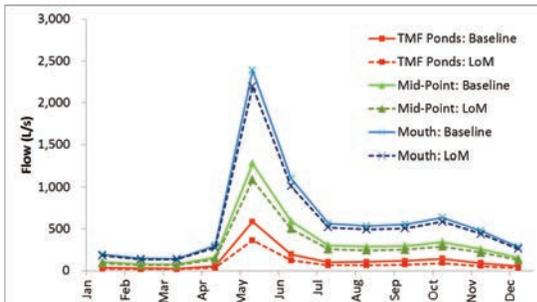
**Fig. 5** Baseline and life of mine (LoM) flow in the Niesajoki River, downstream of the TMF
