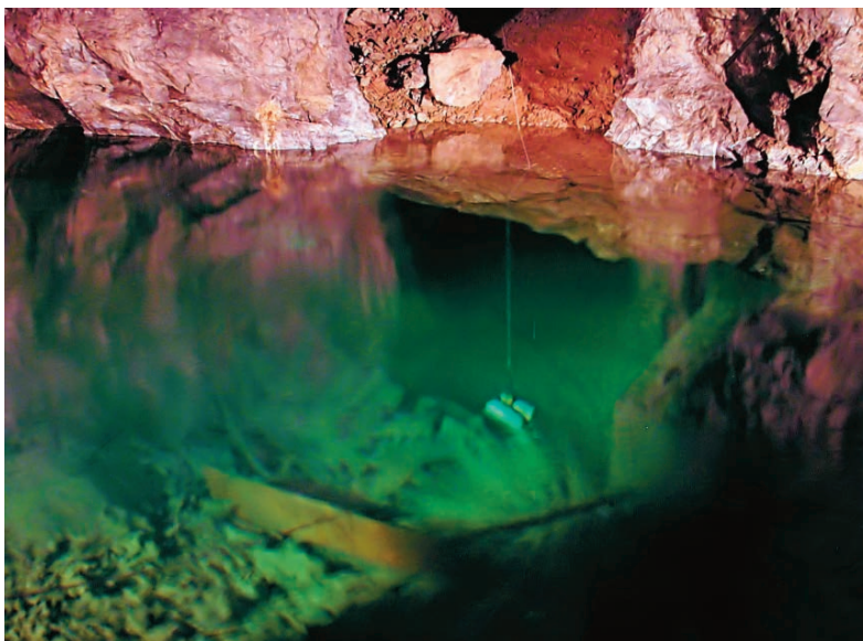
Fig. 4 Tracer probe in the Grüne Grotte incline. The green colour of the water is from the uranine still in the mine water.
