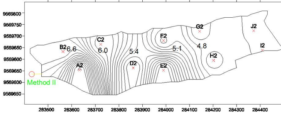
Fig. 6 pH distribution measured in November 2013 at 5 m depth below water level
