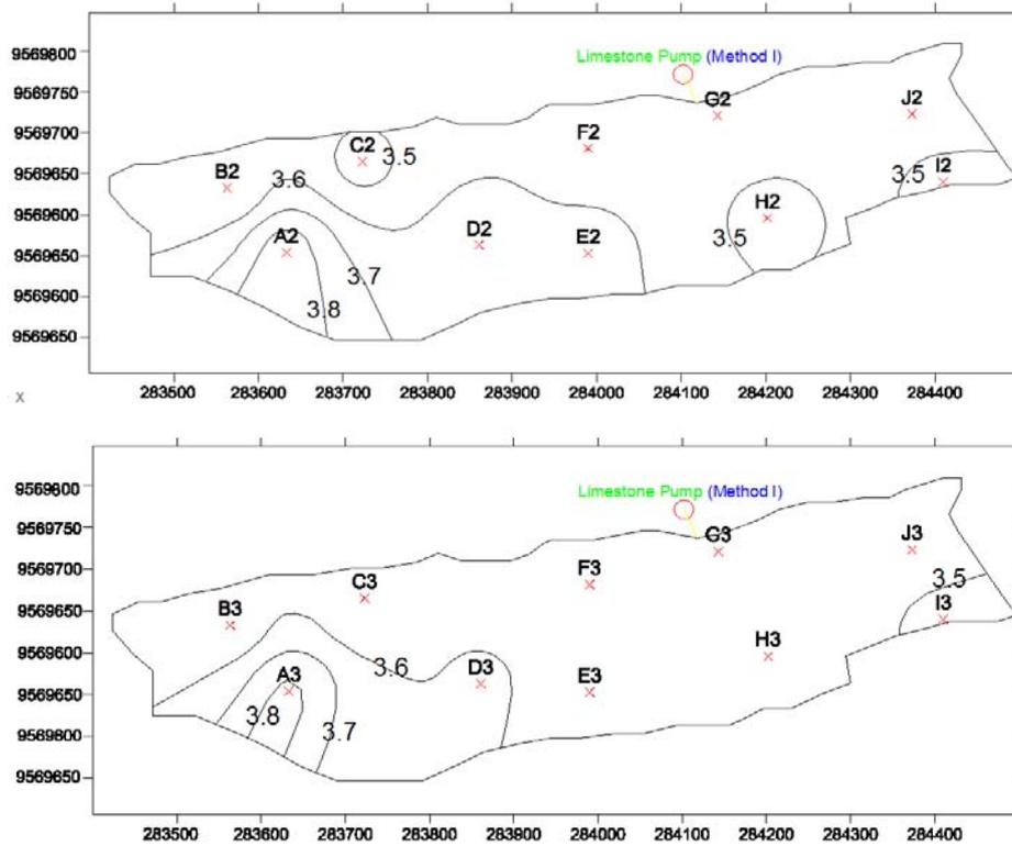
Fig. 5 pH value distribution at 5 m (above) and 10 m (below) depth below water level
