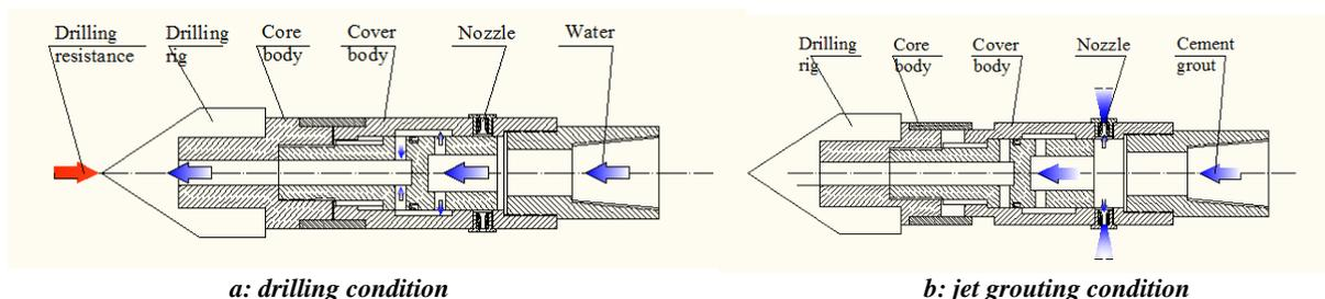
*Fig. 1 Drilling-jetting integrated tool schematic*
