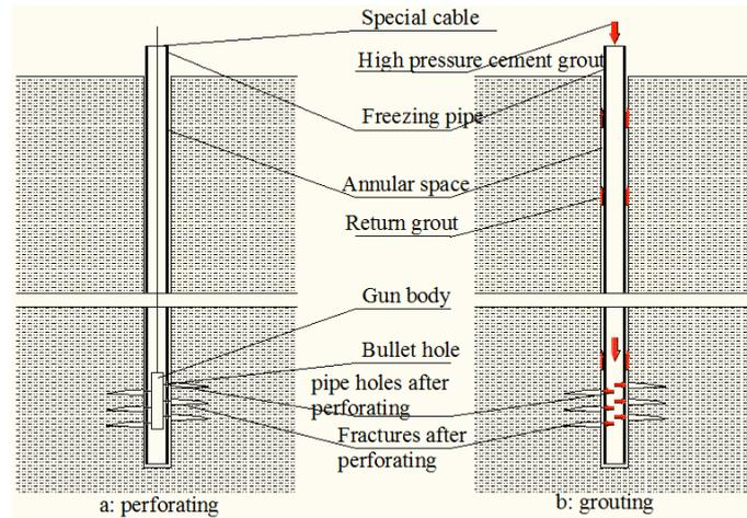
**Fig. 4** Perforating grouting principle schematic
