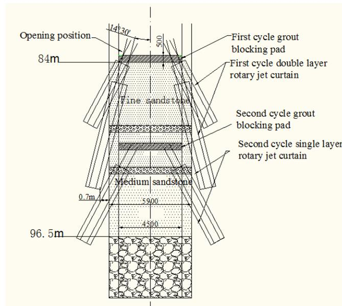
**Fig. 3** Double cycle rotary jet grouting curtain schematic
