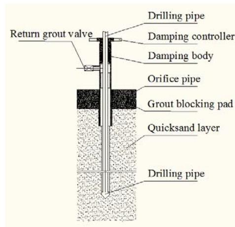
*Fig. 2 grout protected orifice device schematic*
