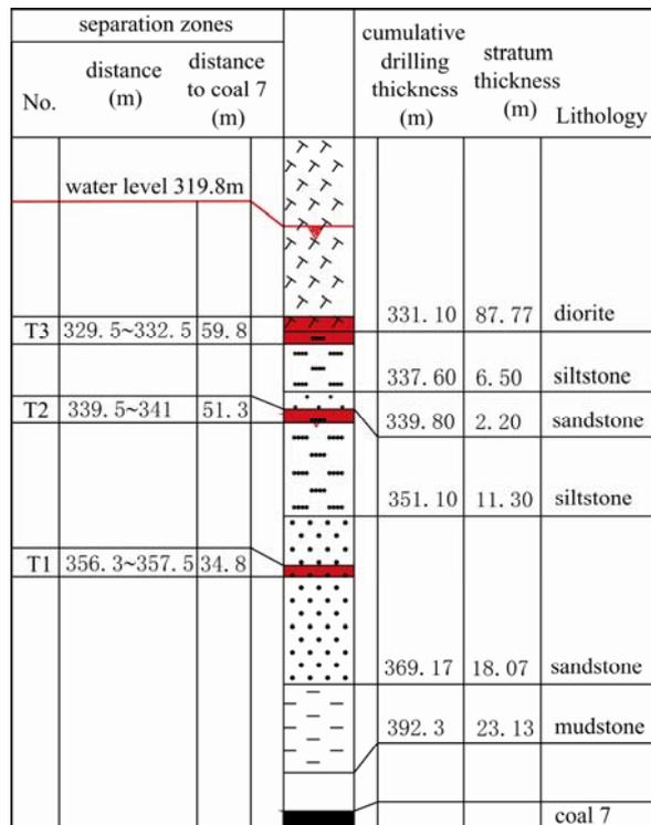
Fig. 3 The position of separation zones by flow rate logging results in borehole R455
