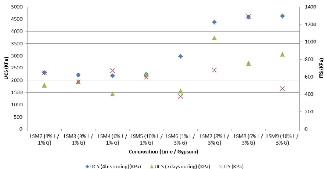
**Fig. 1** UCS (4 hours and 7 days curing) and ITS values for different samples.
