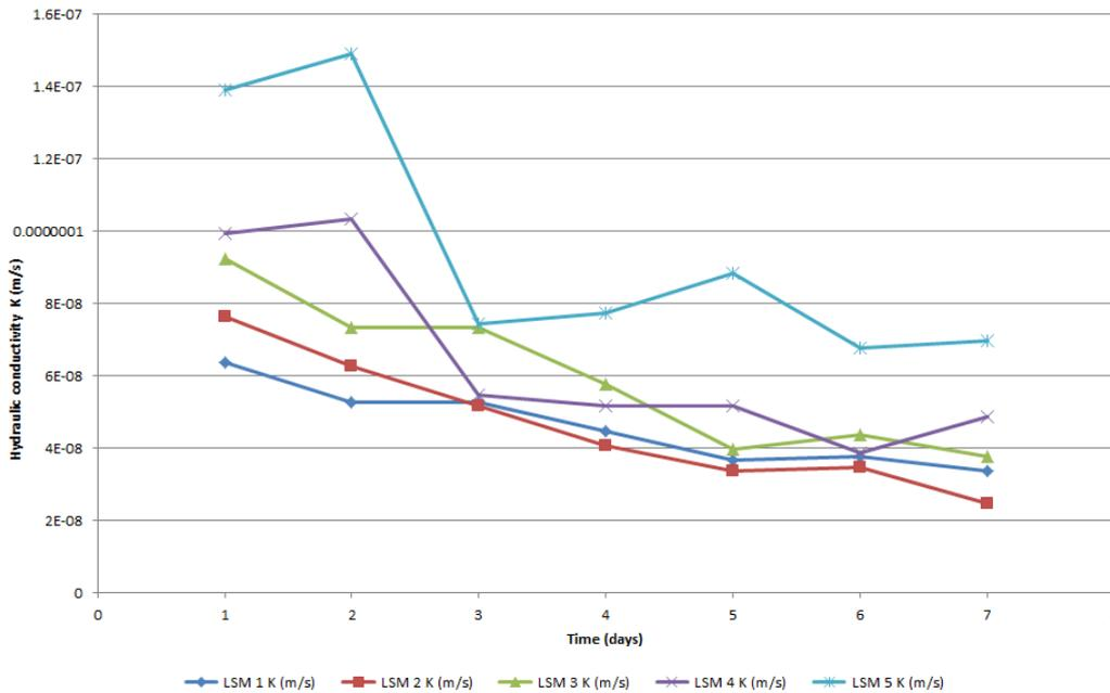
Fig. 2 Hydraulic conductivity (m/s) changes over time for admixtures with 1% gypsum.
