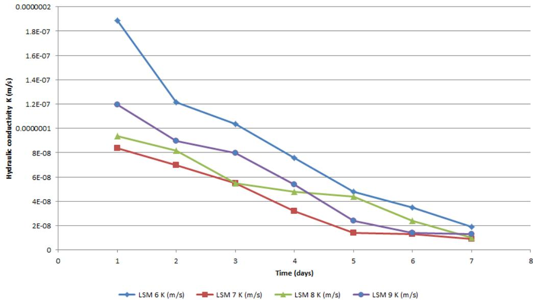
**Fig. 3** Hydraulic conductivity (m/s) changes over time for admixtures with 3% gypsum.
