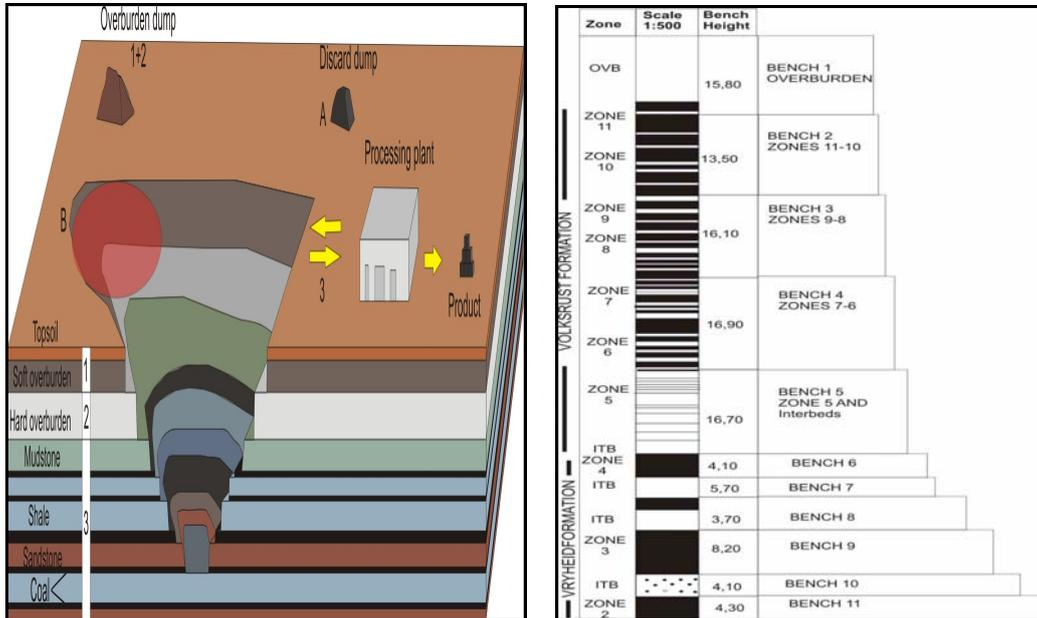
**Fig. 1** Open cast mining in the study area illustrating the waste generated at various phases during mining (Left); Stratigraphic column with the lithological units and benches mined in the Waterberg Coalfield (Right). OVB- overburden and ITB- interburden (Dreyer 1999).
