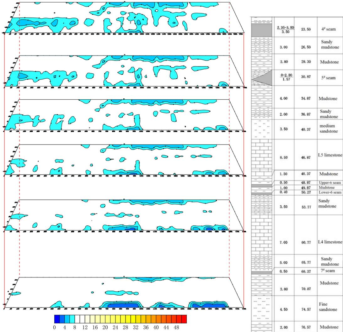
Fig.3 The 3D spatial distribution of anomalies at different depths above the No.80101 workface
